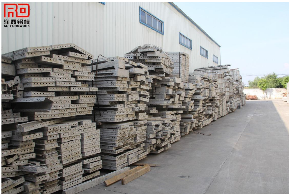
Recycled aluminum formwork standard panels from our domestic building project.
